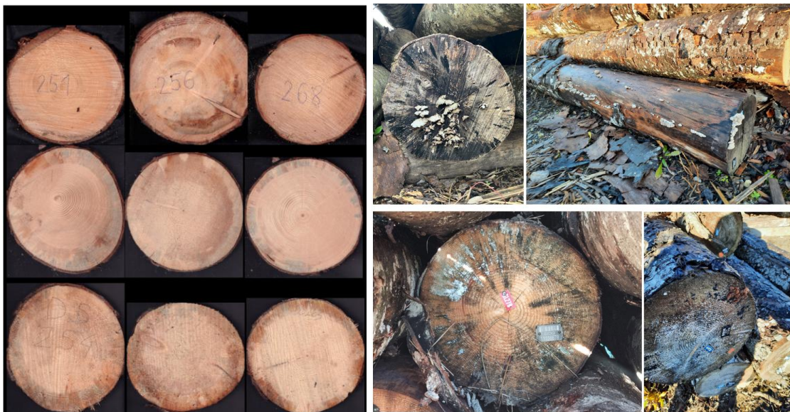
Figure 3. Cross sections of spruce logs and the visual appearance of the logs after nine months
